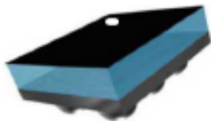
Chip scale package on glass 8 bumps
